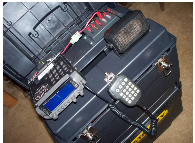
Flip caddy over, attach head and mic and coax. Settle caddy back into the top. Plug in the battery power to the RigRunner.
