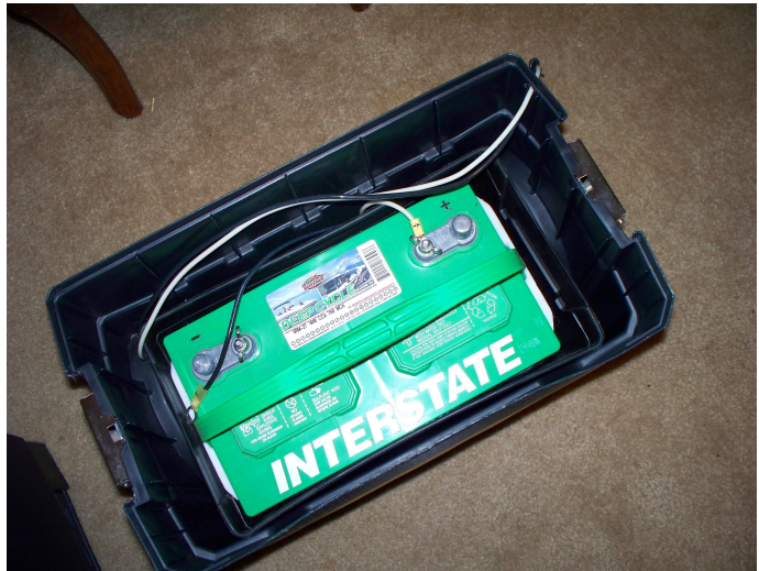
Remove top half of toolbox. Connect power lines. Return top half of toolbox.
